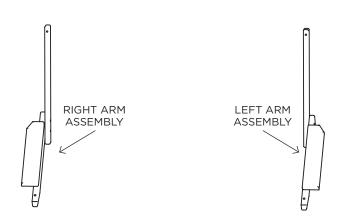
**STEP 2.** Attach upper seat EYE bar to left and right verticals **BOLT** with shorter end of chain sets. WASHER Attach middle chain short eye bolts to left and right arm. (Cushion not pictured.) RIGHT LOCK NUT **VERTICAL UPPER ROPE** RIGHT ARM ← SEAT BAR SHORT ∠ CHAIN ← LEFT VERTICAL LEFT ARM \*
